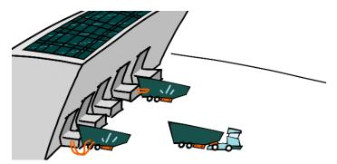
With the **Powerbank-trailer**, part of the batteries is transferred to the trailer. These batteries can be charged independently of the tractor. By coupling the trailer, the energy can be transferred from the trailer to the tractor during driving. This increases flexibility in energy management.
